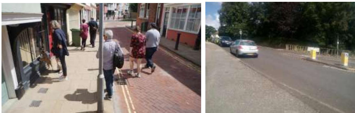
Figure 7-3: Example of narrow footway (Left – West Street) and Pedestrian crossing away from desire line (Right – Bramble Hill Road)
